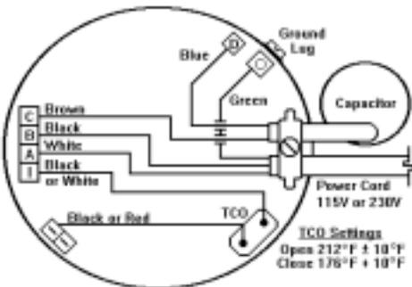
Figure 4 - Wiring Diagram for SM-909 and SM-1212 Models
