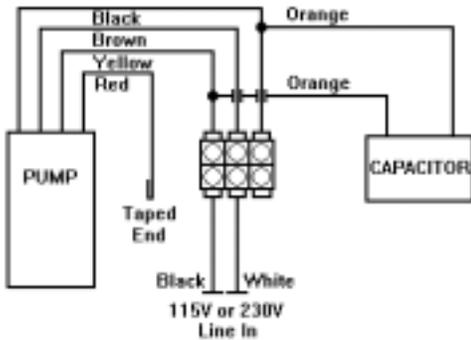
Figure 3 - Wiring Diagrams for SM-303 Models
