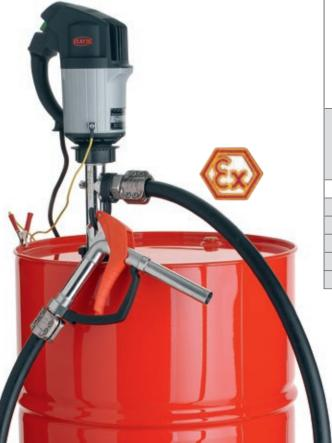
Delivery rate max. 52.8 GPM, delivery head max. 31.1 ft.\* When using the pump with a discharge hose and a hand tap, the delivery rate will be approx. 13.2 GPM.
