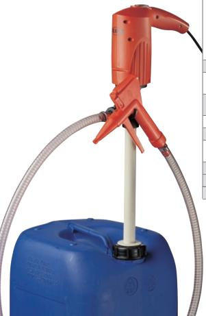
For transferring acids like boric acid, fruit acids, phosphoric acid, hydrochloric acid and sulphuric acid (at 80 %). Delivery rate max. 12 GPM, delivery head max. 22 ft.\* When using the pump with a discharge hose and a hand tap, the delivery rate will be approx. 7.9 GPM.
