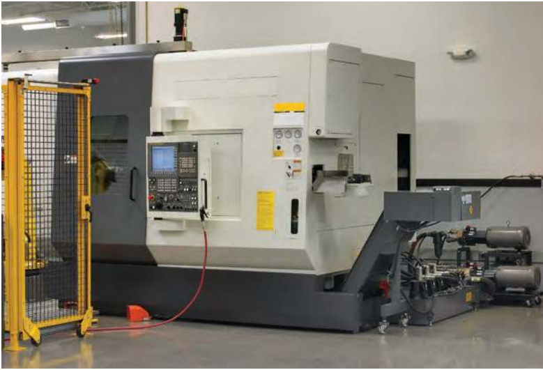
Three Hydra-Cell model D10 pumps deliver high-pressure coolant for a turret-type, multi-tasking boring machine with 16 tool stations for bar work and 12 tool stations for chuck work.
