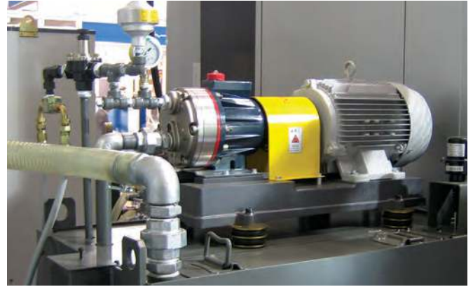
Unlike pumps that decrease flow significantly as pressure increases, Hydra-Cell flow rates are proportional to the pump speed. Delivery of the machine tool coolant can remain at a consistent high pressure while pump flow is set for the rate best suited to the machine tool in use.
