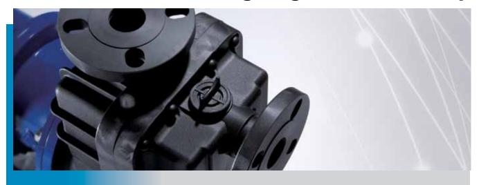
SMX Series of magnetically driven non-metallic pumps offer an innovative true self-priming design with no mechanical seals for years of trouble-free service. SMX features our self-radiating bearing structure and our proven non-contact dry-run capability enabling them to withstand the rigors of abnormal operating conditions. Utilizing an integral priming and air separation chamber, the SMX Series offer superior repeatable self-priming performance.
