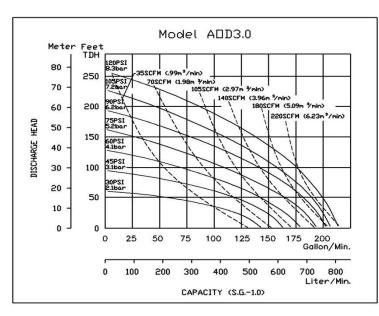
The performance curves shown and other published literature reflect an average performance for all materials and all elastomers, including Teflon®. Derating of the performance is not necessary for Teflon® fitted pumps.
