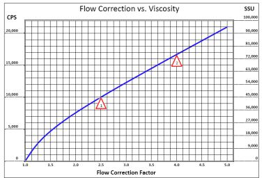
To determine the correction flow rate, find the intersection of the VISCOSITY on the above curve and read the FLOW CORRECTION FACTOR. Multiply this factor by the desired flow of the pump and use this new flow rate to select a pump from the performance curves.
