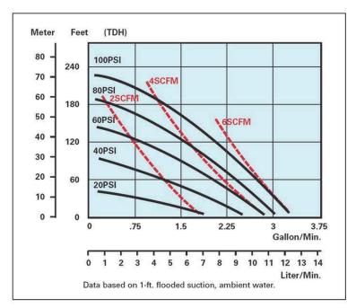
The performance curves shown and other published literature reflect an average performance for all materials and all elastomers, including Teflon®. Derating of the performance is not necessary for Teflon® fitted pumps.
