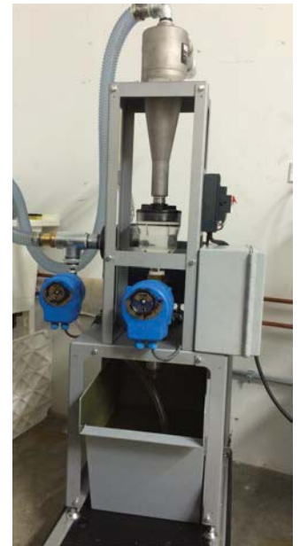
Example 1: Modified C-SEL with electrical actuated valves and sludge tank.
